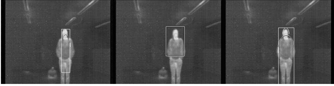
Fig. 10. Comparing elliptic measurement (left), feature model (middle) and combination (right).
